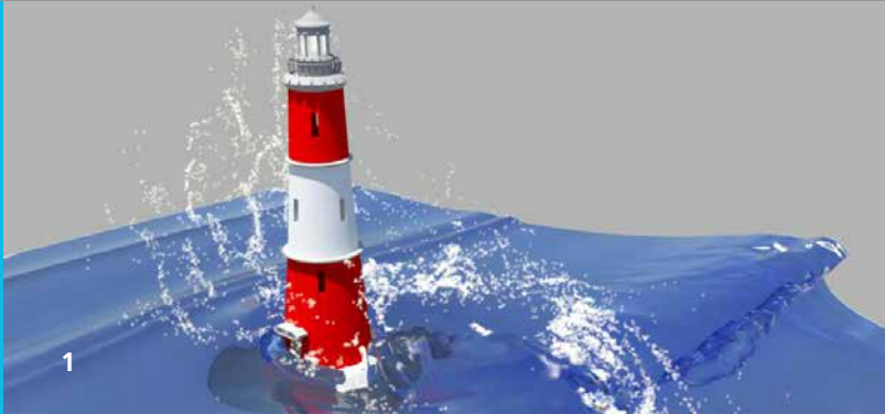
1 Two-phase fluid flow with coupled particle droplets © M. Griebel, P. Zaspel (INS, University of Bonn)
